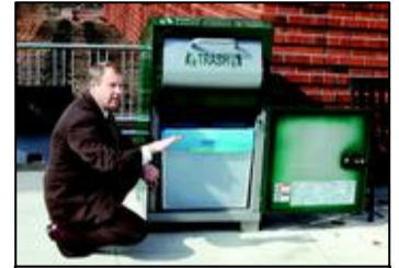
Bill Eddy, director of sales for New England for Seahorse Power Co., shows off the first solar powered trash compactor on Cape Cod at Cape Cod Community College. The BigBelly solar compactor has a 40-watt solar panel, which powers the compactor. (Rich Eldred)
