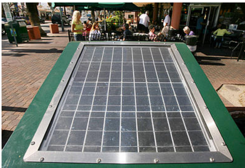
LEFT: The city is testing four compactors that use the sun's energy to compress garbage into 40-pound bricks, reducing trash collection.
